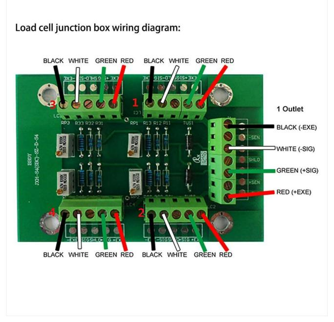
Figure 3: Load Cell Junction Box Wiring Diagram
