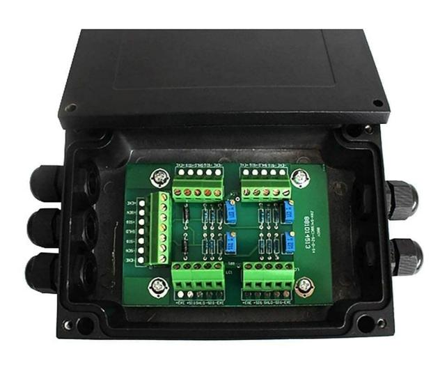
Figure 4: Internal View of Junction Box
