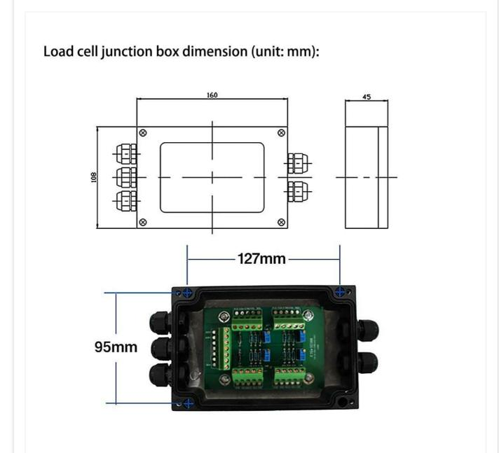
Figure 2: Load Cell Junction Box Dimensions
