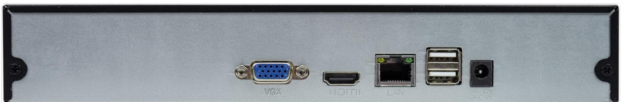
Image: Rear view of the PNI House IP516 NVR, displaying VGA, HDMI, LAN, USB, and DC 12V power input ports.
