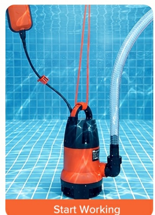
Immerse the Pump in Water at an Angle to Allow Any Trapped Air to Escape.
