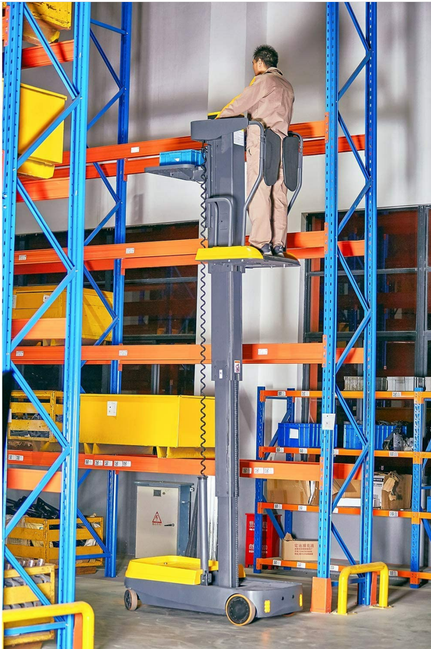
Figure 6.3: An operator utilizing the Xilin Mini Order Picker to access items on high shelving in a warehouse environment.
