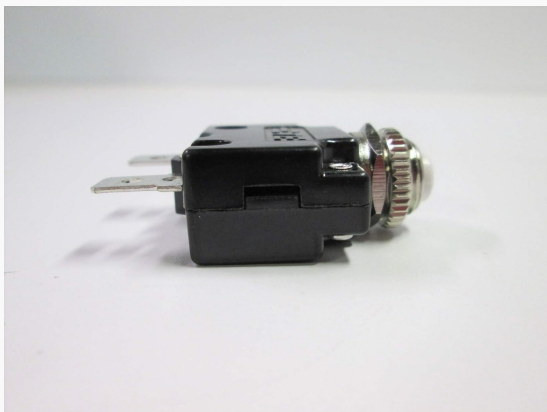
Figure 3.3: Side profile of the circuit breaker. This view emphasizes the compact dimensions of the unit and the threaded portion of the mounting post.
