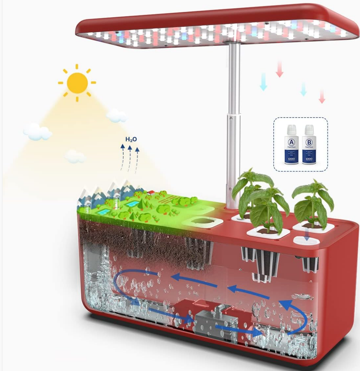
Figure 3: Illustration of the hydroponic circulation system and nutrient application.
