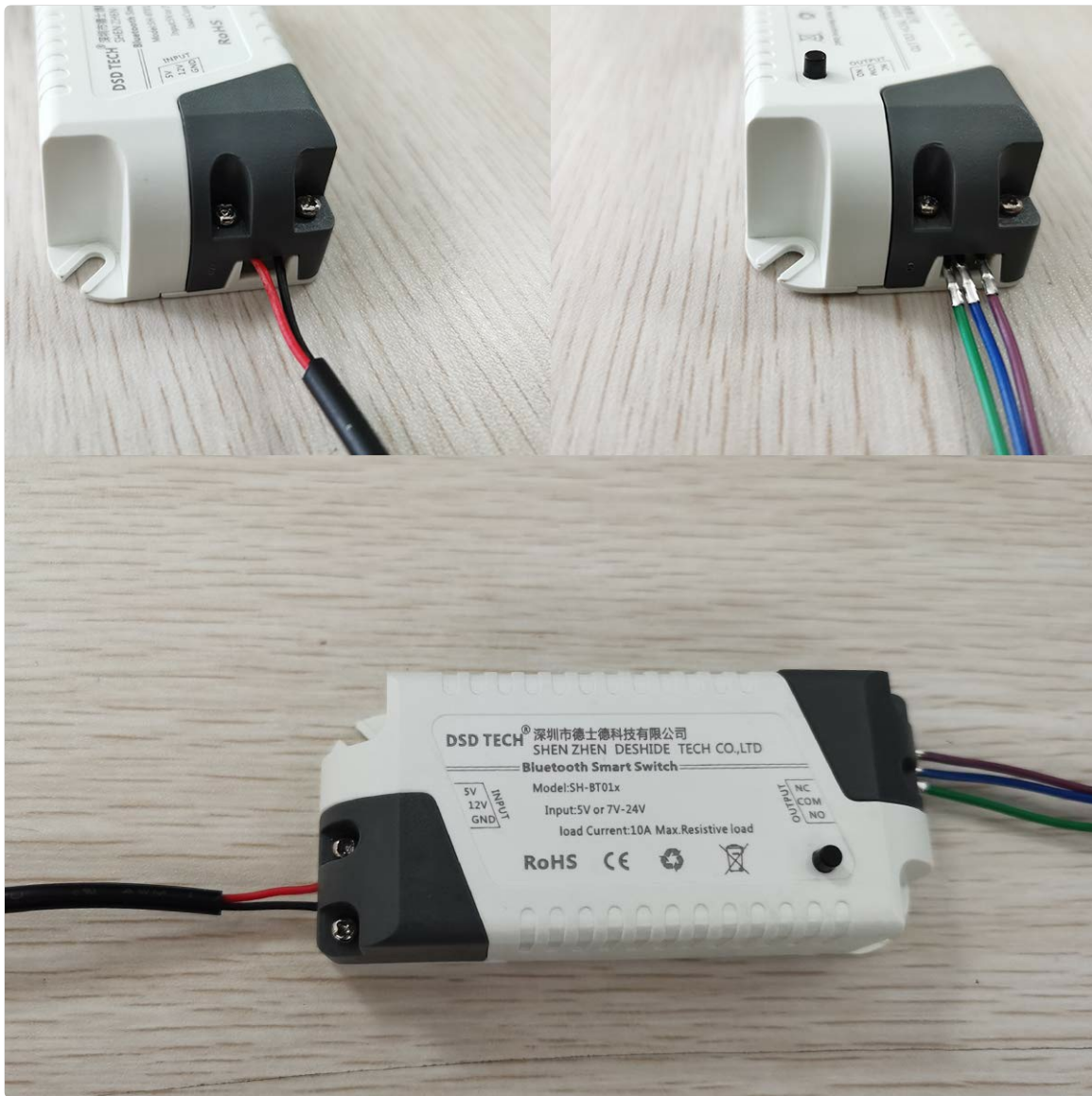
Figure 4: Wiring Example. This image illustrates how to connect power and load wires to the relay module's terminals.
