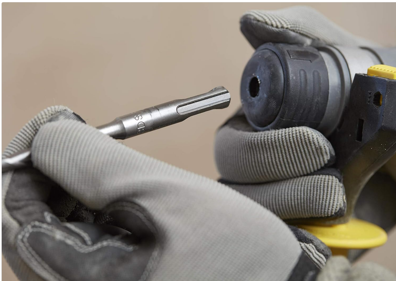
Figure 6: Inserting an SDS-Plus drill bit into the tool's chuck.
