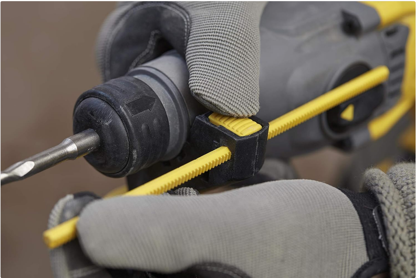
Figure 7: Adjusting the depth stop for controlled drilling depth.
