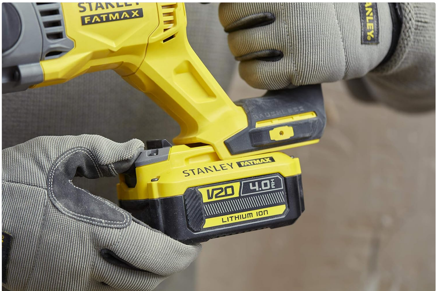
Figure 3: Proper method for inserting the battery pack into the tool's base.
