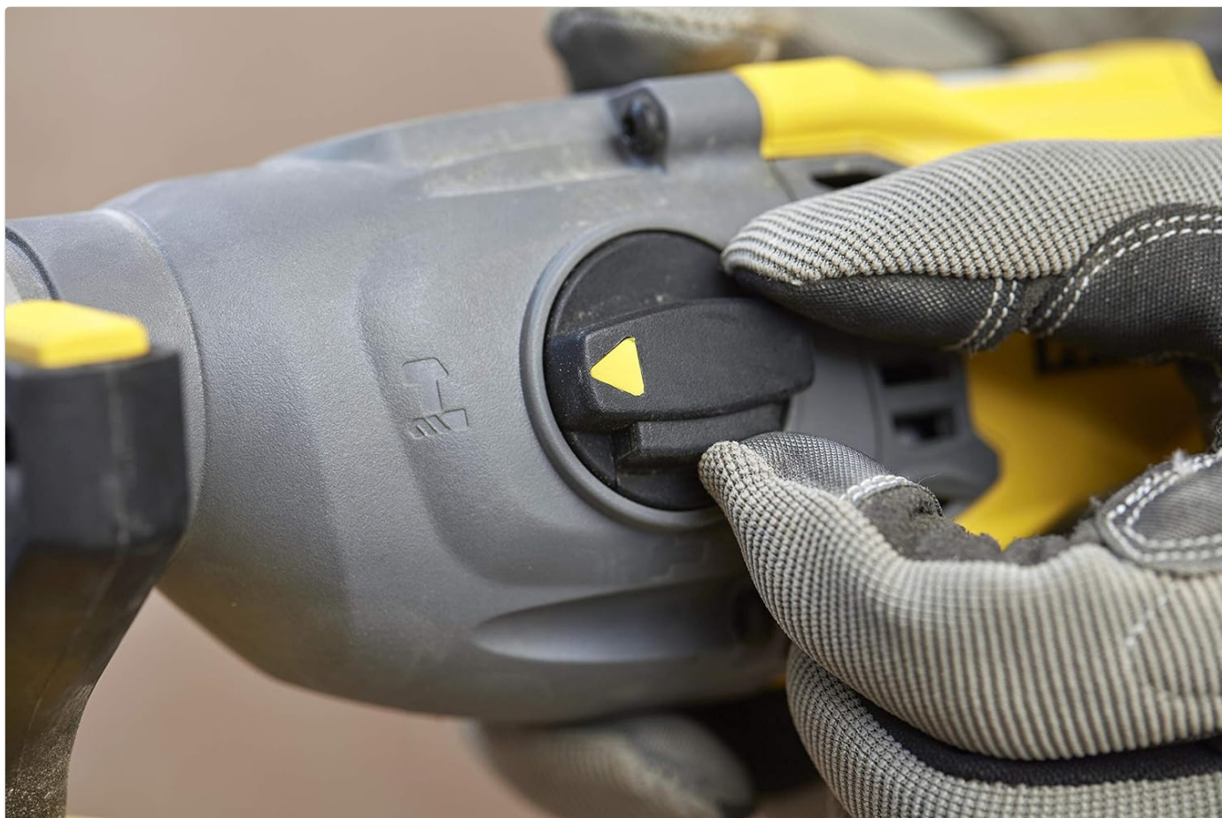
Figure 8: The mode selector switch allows selection of drilling, hammer drilling, or chiseling functions.
