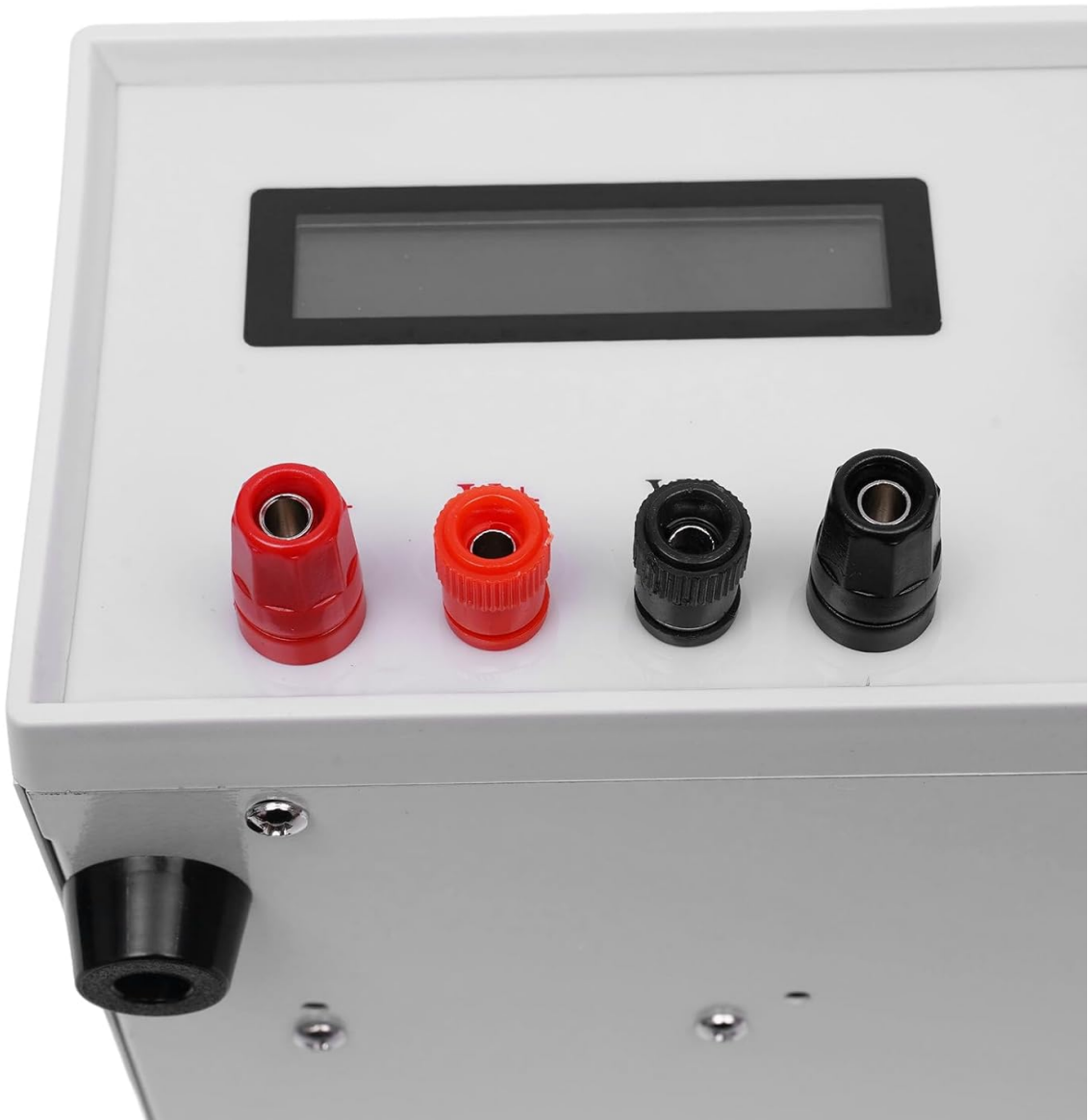
Image 4.2: Close-up view of the A+, V+, V-, and A- terminals.
