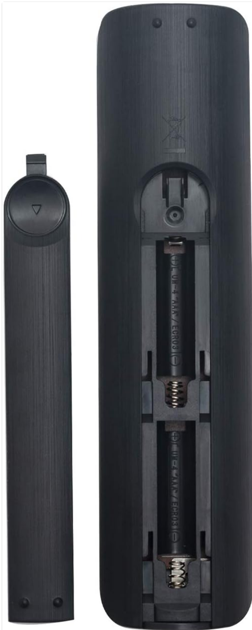
Figure 2: Back view of the remote control with the battery compartment open, illustrating correct battery placement.
