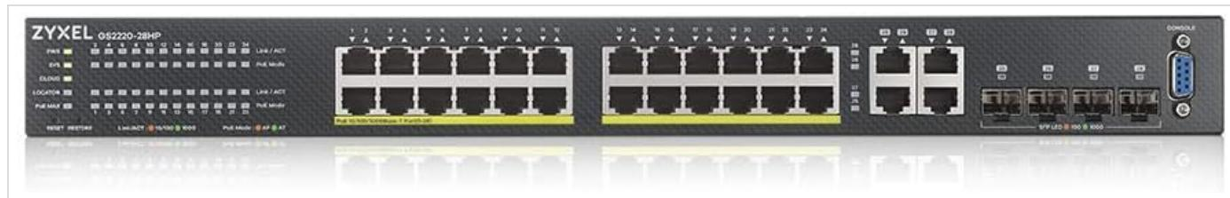
The front panel of the GS2220-28HP switch displays the 24 Gigabit Ethernet ports, four combo RJ-45/SFP ports, and two additional SFP ports. It also includes various LED indicators for power, system status, link/activity, and PoE status for each port. A console port is located on the far right for direct management access.
