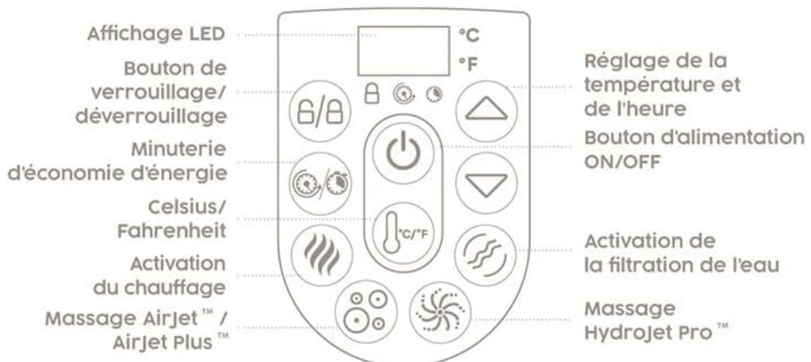
Figure 6: Digital control panel layout. This diagram labels each button and indicator on the spa's control panel, including
