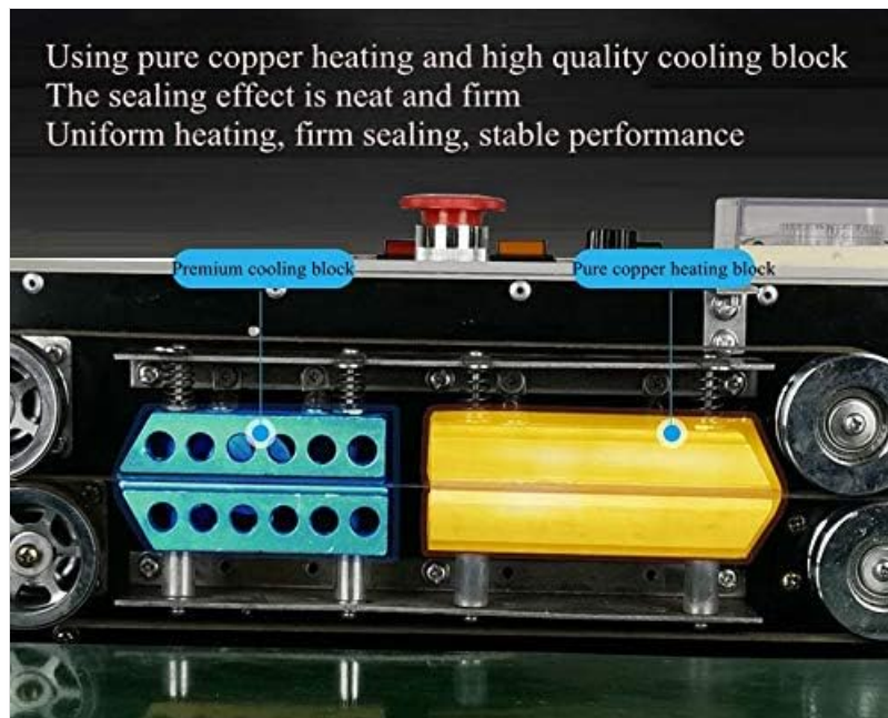
Figure 3.4: Internal view of the sealing area, illustrating the heating and cooling blocks.
