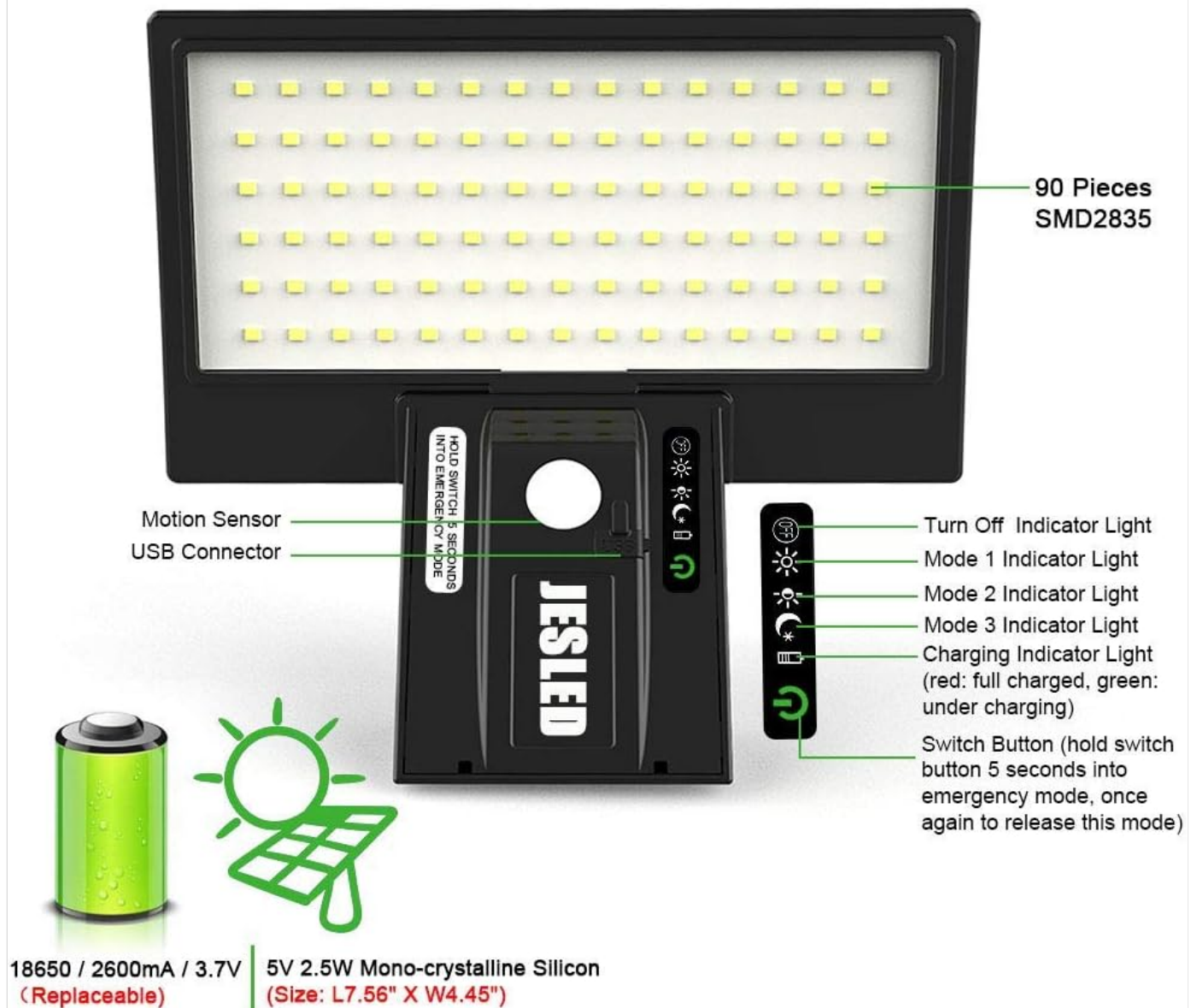
Figure 2: Key Components of the Solar Flood Light
