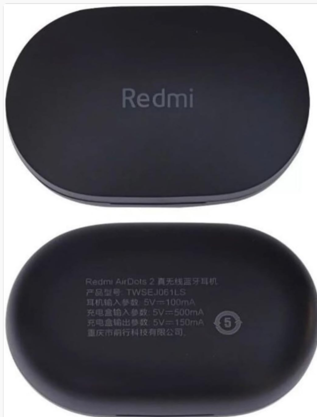
Image: The bottom of the charging case, displaying product information and specifications in Chinese, including model number TWSEJ061LS.
