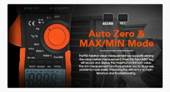
This image illustrates the 'Auto Zero & MAX/MIN Mode' functions. The "REL" (relative value) key allows users to zero out a reading before measurement. The "MAX/MIN" key records and displays the maximum or minimum measured values, aiding in diagnosing problems and improving troubleshooting efficiency.
