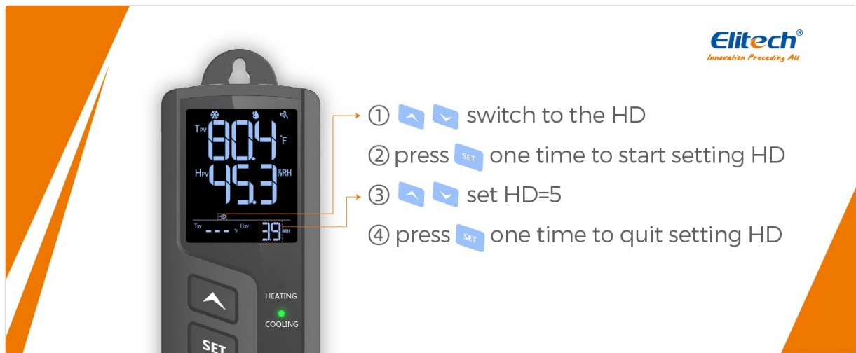
Figure 4: Detailed steps for setting humidity parameters (HS and HD) on the controller.
