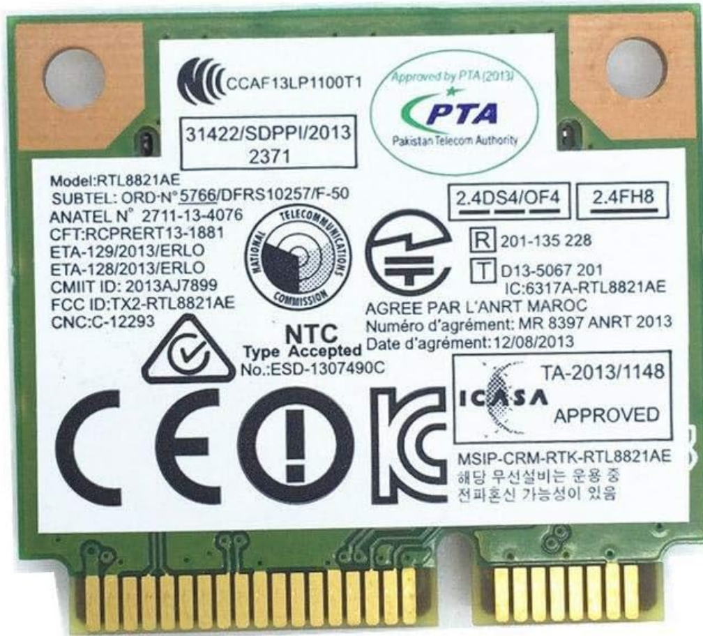
Figure 2.2: Back view of the Realtek RTL8821AE card. This image shows the underside of the card, featuring multiple international regulatory compliance logos and certifications such as CE, FCC, and PTA, indicating its adherence to various global standards.
