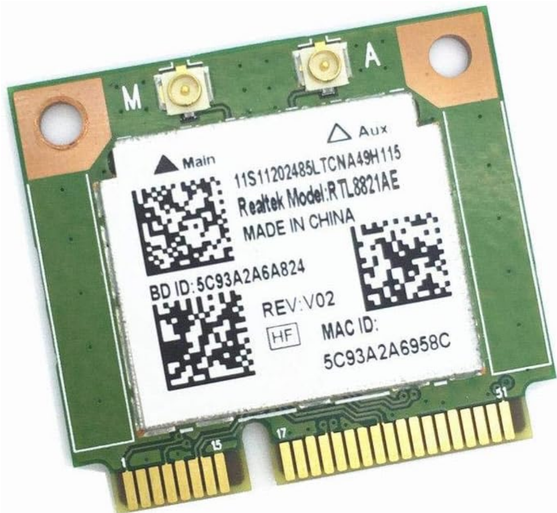
Figure 2.1: Front view of the Realtek RTL8821AE card. This image displays the top side of the Half Mini PCI-e card, featuring the Realtek RTL8821AE chip, two antenna connectors labeled 'Main' and 'Aux', and various identification markings including QR codes and model number.
