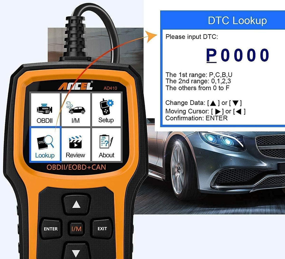
Image: The ANCEL AD410 screen showing the DTC Lookup interface, prompting the user to input a code.
