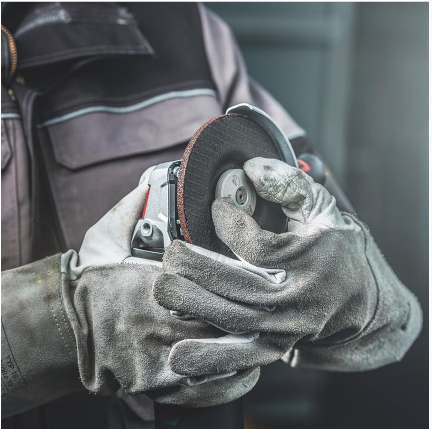
Figure 3: Demonstrating the tool-free disc change using the M-Quick system.
