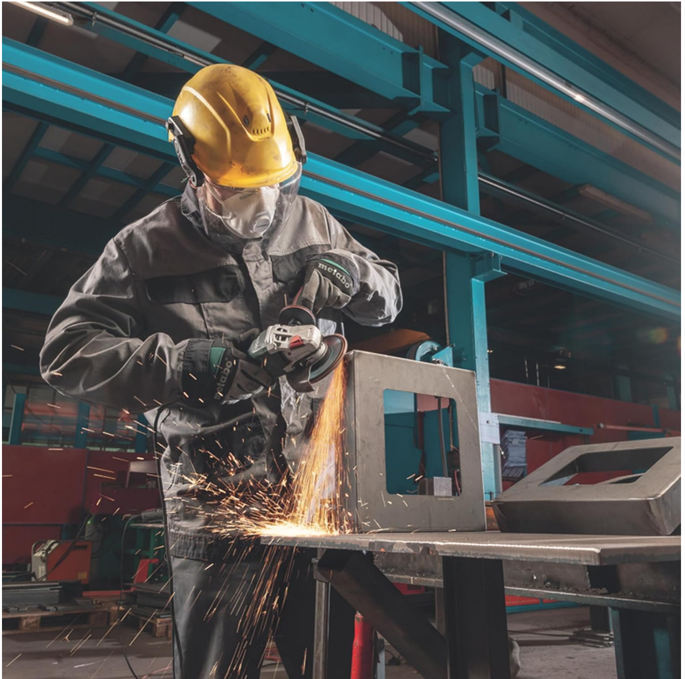
Figure 4: Proper technique for grinding, showing sparks being safely directed.
