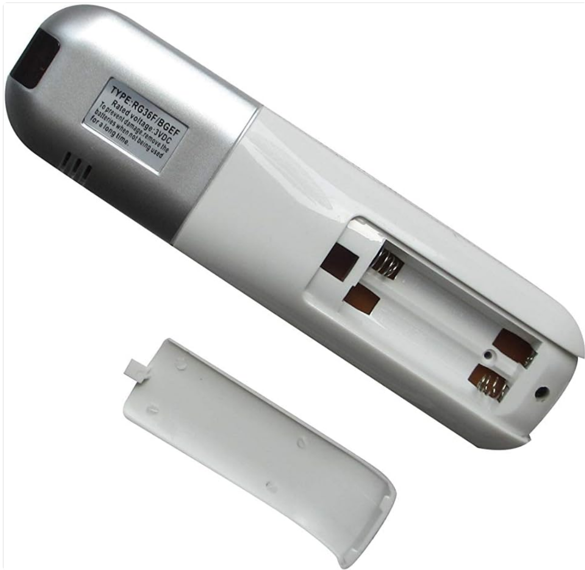
Image: Back view of the remote control with the battery cover removed, illustrating the battery compartment where two AAA batteries are to be inserted.
