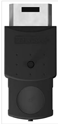
Image description: A close-up view of the Sega Saturn port receiver, which connects the wireless controller to a Sega Saturn console.
