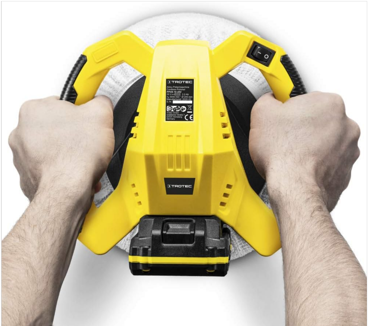
Figure 3: Proper two-hand grip for operating the polisher, ensuring control and stability.
