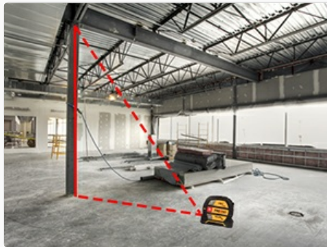
Image 5.6: Illustration of the 2-point Pythagorean measurement mode for indirect height calculation.
