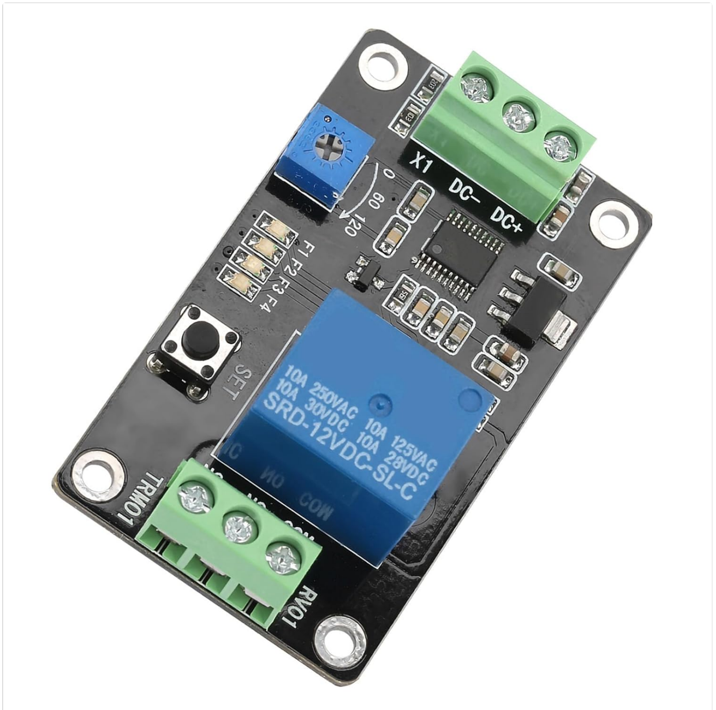
Figure 2: Overhead view highlighting the function selection labels (F1, F2, F3, F4) and the time adjustment potentiometer markings (0, 60, 120 seconds).
