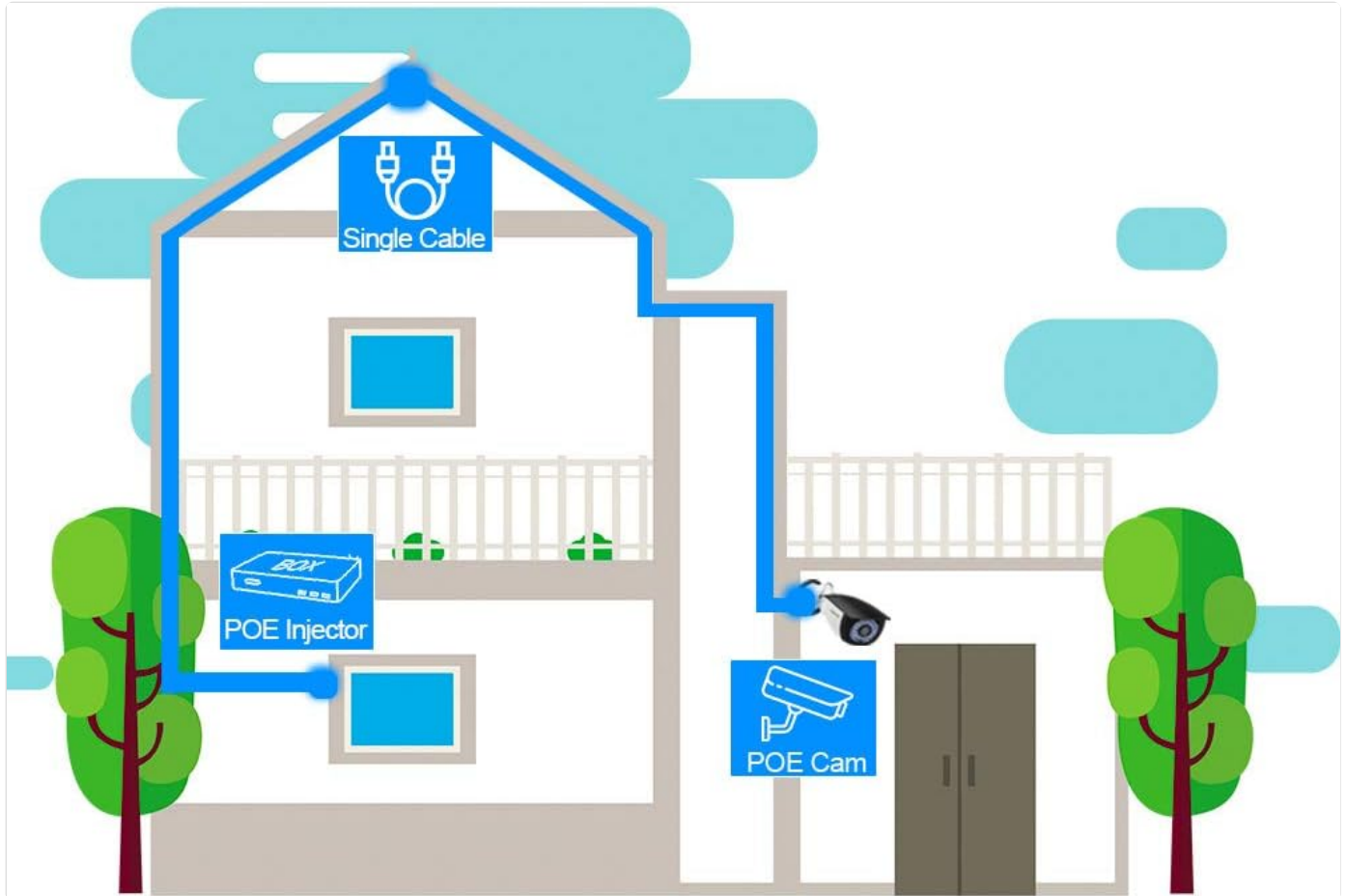
Image: An illustration demonstrating the Power Over Ethernet (POE) setup. A single Ethernet cable runs from a POE injector (connected to a router) to the POE camera, providing both power and network connectivity.
