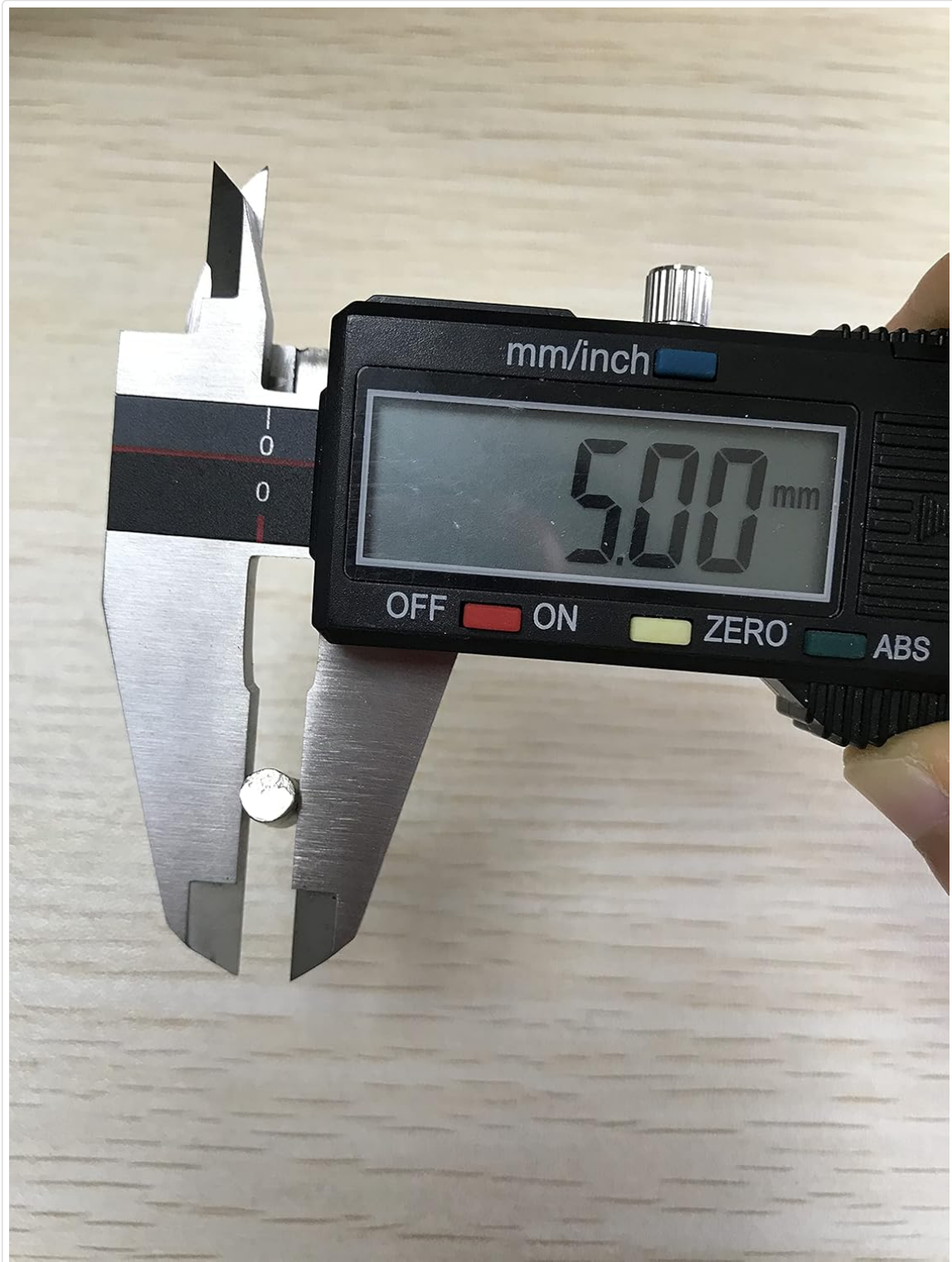
Image 4.1: Measuring a shelf peg to confirm 5mm diameter. Accurate measurement ensures proper fit.
