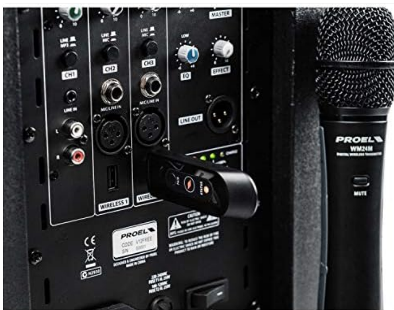
Figure 4.3: A close-up view of the USB port on the Proel V12FREE, demonstrating how a Proel U24 wireless microphone receiver can be connected for wireless audio input.
