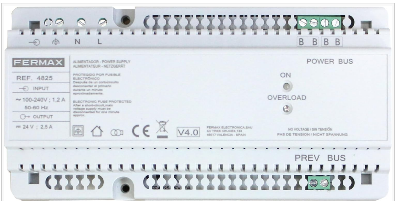
Figure 1: Front view of the FERMAX 4825 DUOX Plus DIN10 Power Supply. The image displays the input terminals (N, L), output terminals (24V, 2.5A), Power Bus and Prev Bus terminals, and LED indicators for ON and OVERLOAD status. Key specifications like input voltage (100-240V; 1.2A, 50-60Hz) and output voltage (24V; 2.5A) are visible, along with the FERMAX brand logo and model
