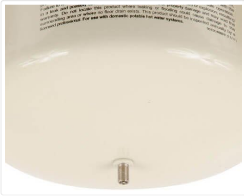
Figure 2: Bottom view of the Amtrol ST-5 expansion tank, highlighting the Schrader valve. This valve is used to adjust the internal air pre-charge pressure of the tank.
