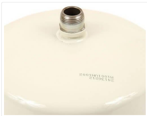
Figure 1: Top connection point of the Amtrol ST-5 expansion tank. This is the 3/4 inch NPT threaded connection for plumbing into the cold water supply line of the water heater.
