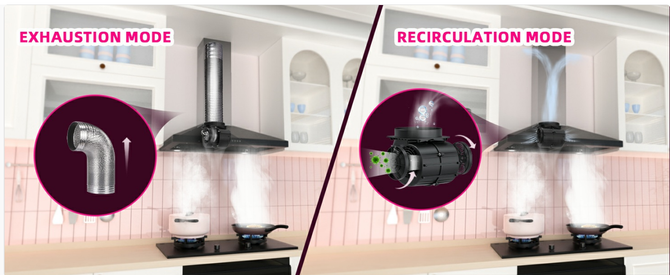
Figure 4: Exhaustion (Ducted) and Recirculation (Ductless) Modes
