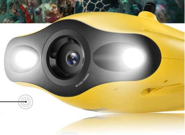
Figure 2: Close-up view of the Gladius Mini's 4K HD camera and dual LED headlights, designed for superior underwater visibility and image capture.
