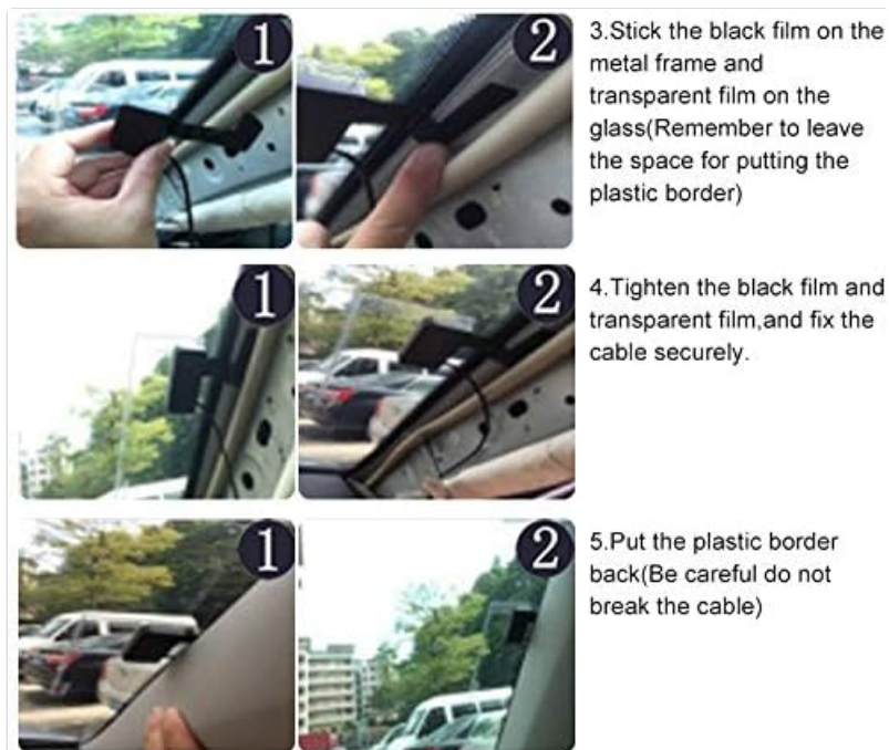
Image 4.1: Step-by-step guide for installing the DAB antenna on your vehicle's window.
