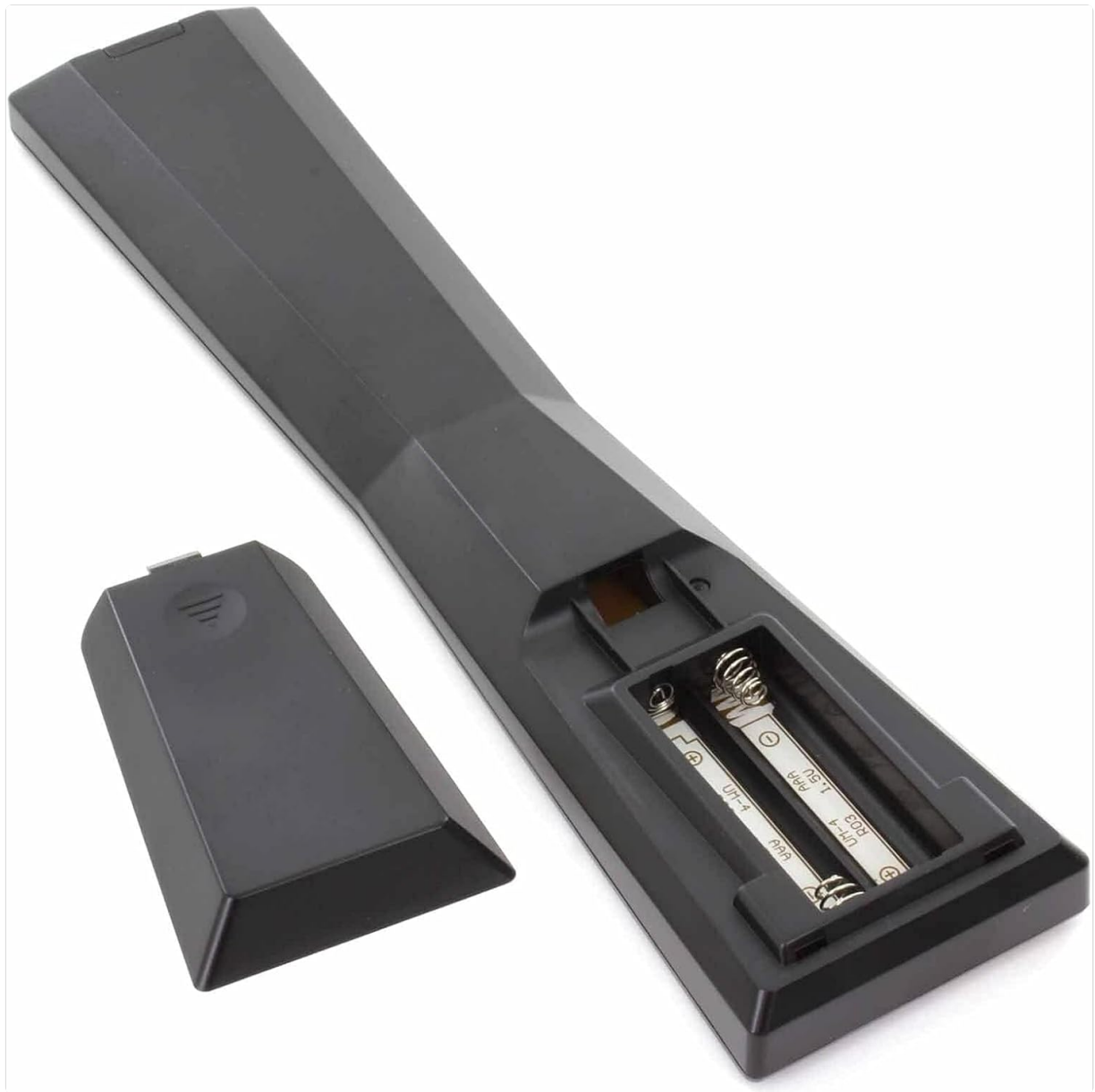
Image: Back view of the JVC RM-C3338 remote control with the battery compartment open, showing the slots for two AAA batteries.
