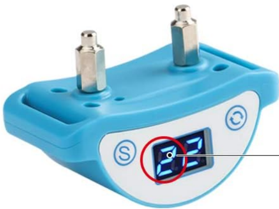
Image 5.2: Illustration of the two sound detection modes, Mode 1 for short meows and Mode 2 for long meows, indicated on the device's display.
