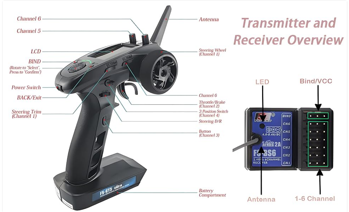
Image 8.1: FS-BS6 receiver highlighting its compact size and built-in gyro.
