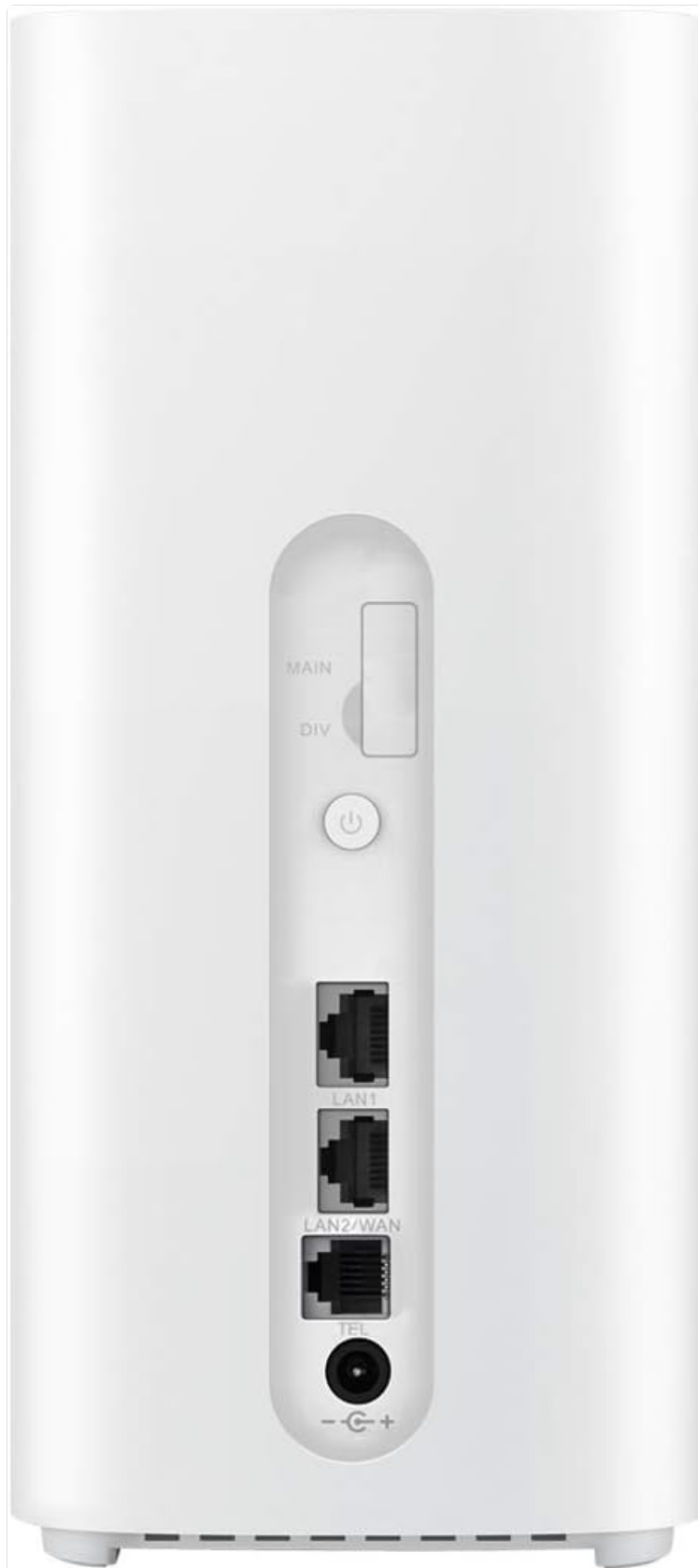
Figure 2: Rear view of the HUAWEI B818-263 router. This image shows the back panel of the router, featuring two TS9 connectors labeled "MAIN" and "DIV" for external 4G antennas, a power button, two RJ45 Gigabit Ethernet ports (LAN1 and LAN2/WAN), an RJ11 telephone port, and the DC power input.
