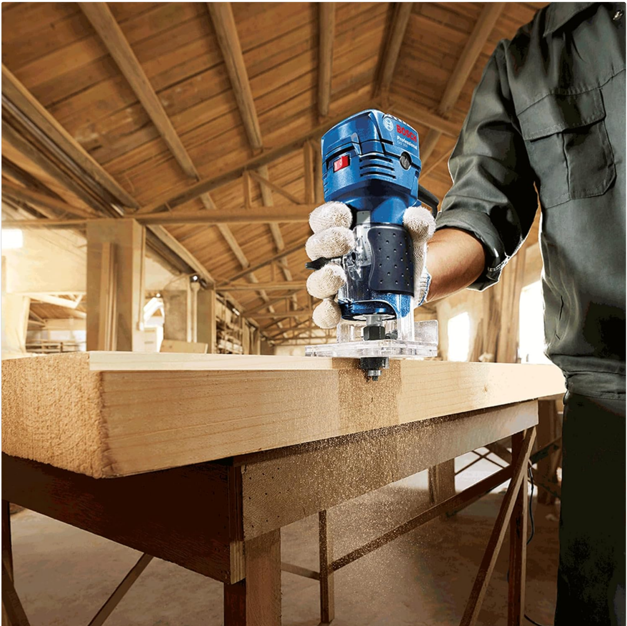
Image 6.1: Proper handling of the Bosch GKF 550 Router during operation.
