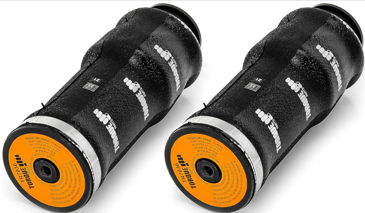
Image: Two TORQUE TR7036 Cab Sleeper Air Spring Bags, showcasing their robust construction and design.
