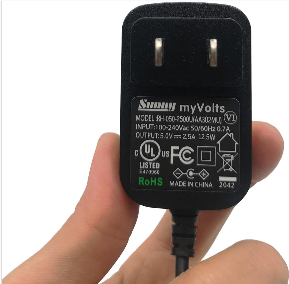
Image 3.1: Detailed view of the power supply label, indicating input (100-240Vac, 0.7A) and output (5.0V, 2.5A, 12.5W) specifications, along with UL, FC, and RoHS certifications.
