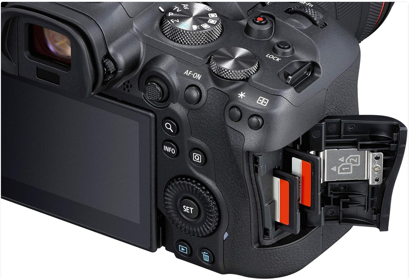
Figure 2.2: Dual UHS-II SD memory card slots on the Canon EOS R6.
