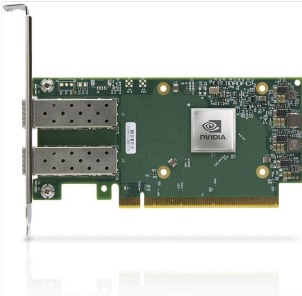
Figure 2: Top view of the Mellanox NVIDIA ConnectX-6 Dx Ethernet SmartNIC, showing the heatsinks and connector ports.
