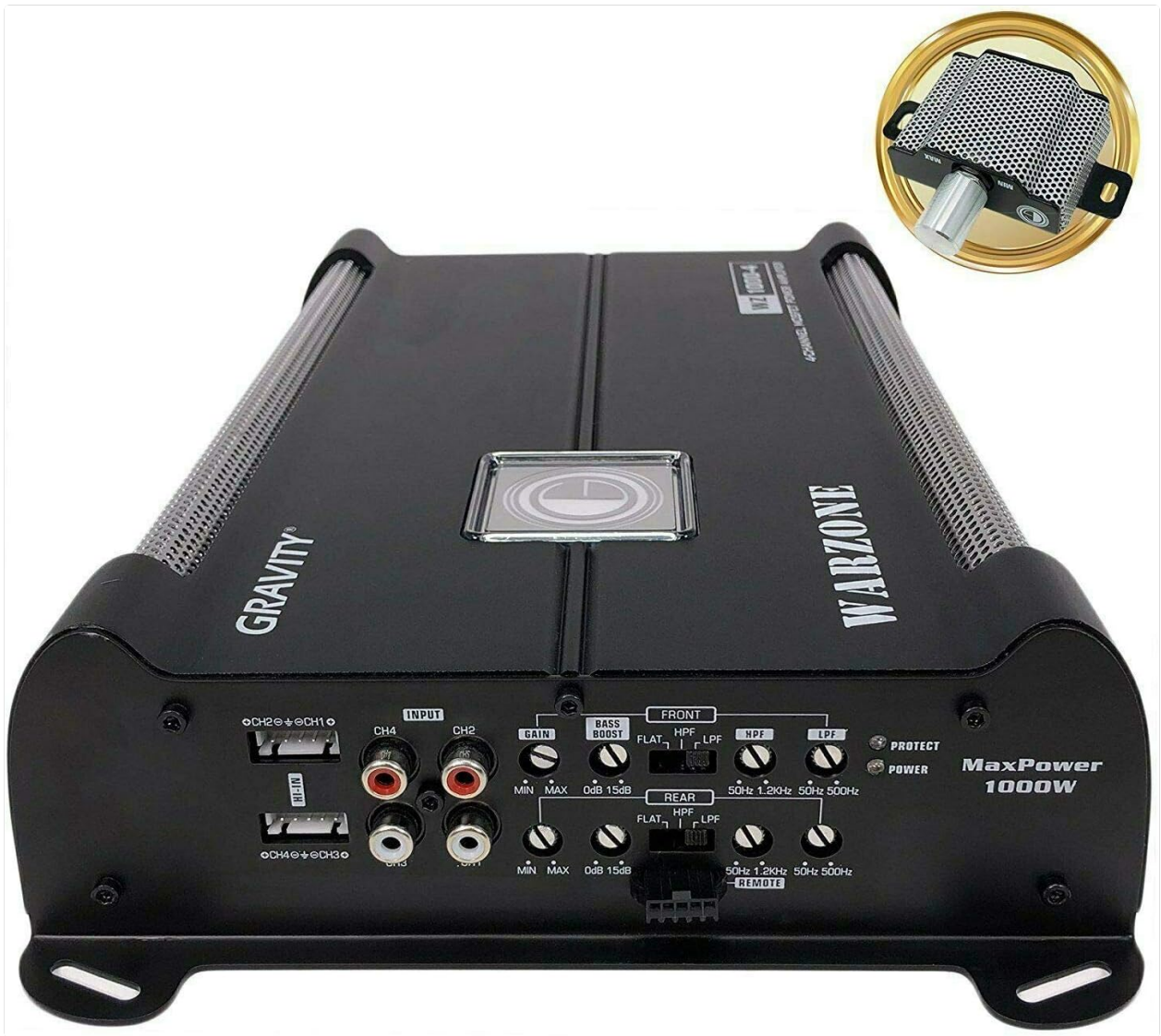
Figure 3.2: Input and control panel of the amplifier, featuring RCA inputs, gain controls, crossover settings (LPF, HPF), and bass boost.
