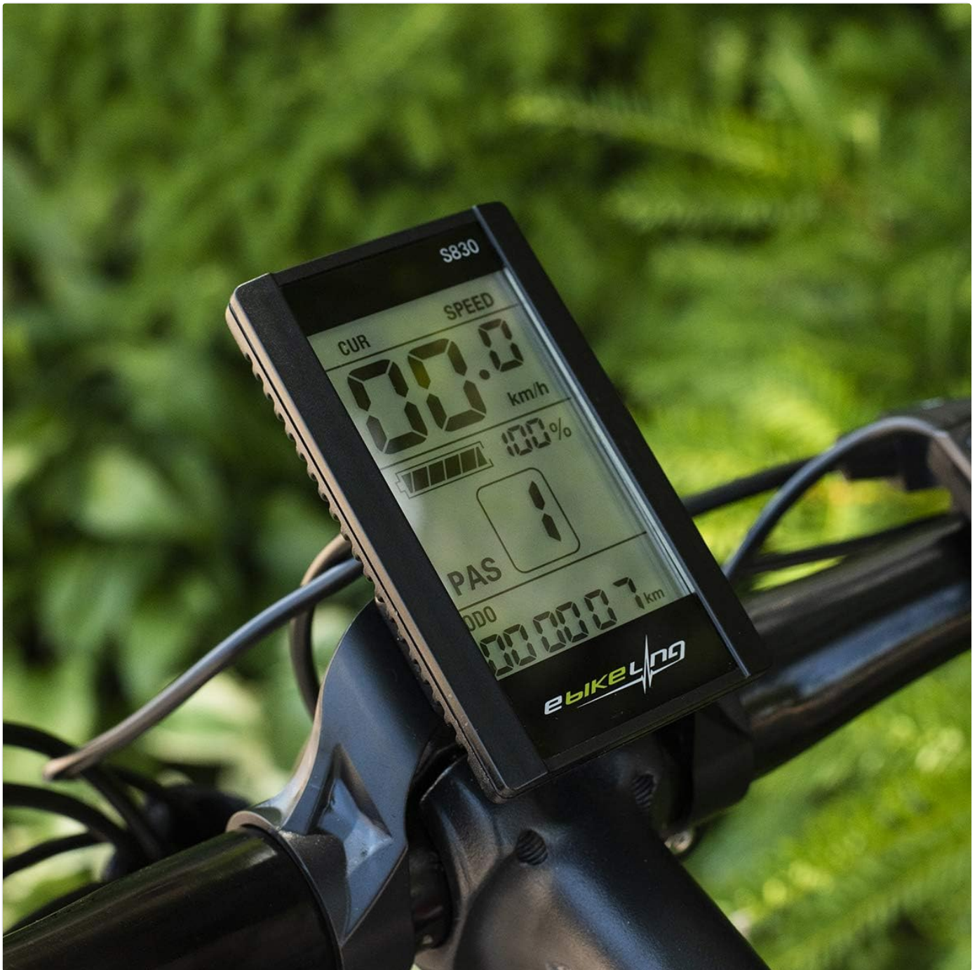
Figure 3: The EBIKELING S830 LCD display mounted on an electric bicycle handlebar, showing its clear screen with speed, battery, and PAS indicators. The image demonstrates the display's readability in an outdoor setting.
