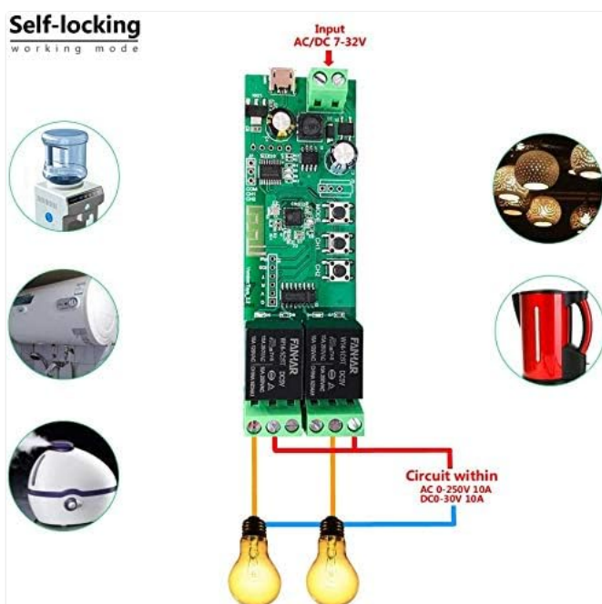
Image 4.3: Wiring for Self-locking mode, ideal for controlling lights or other devices that require a sustained ON/OFF state. Input power can be AC/DC 7-32V.
