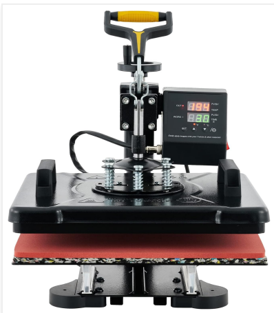
Figure 2: Front view of the heat press machine, showing the main platen and control panel.
