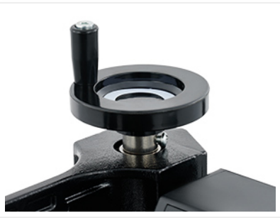
Figure 4: The pressure adjustment knob, located at the top of the machine, used to modify pressing force.
