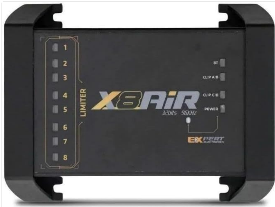
Figure 1: Front view of the EXPERT X8AIR Digital Sound Processor, showing the limiter indicators and branding.
