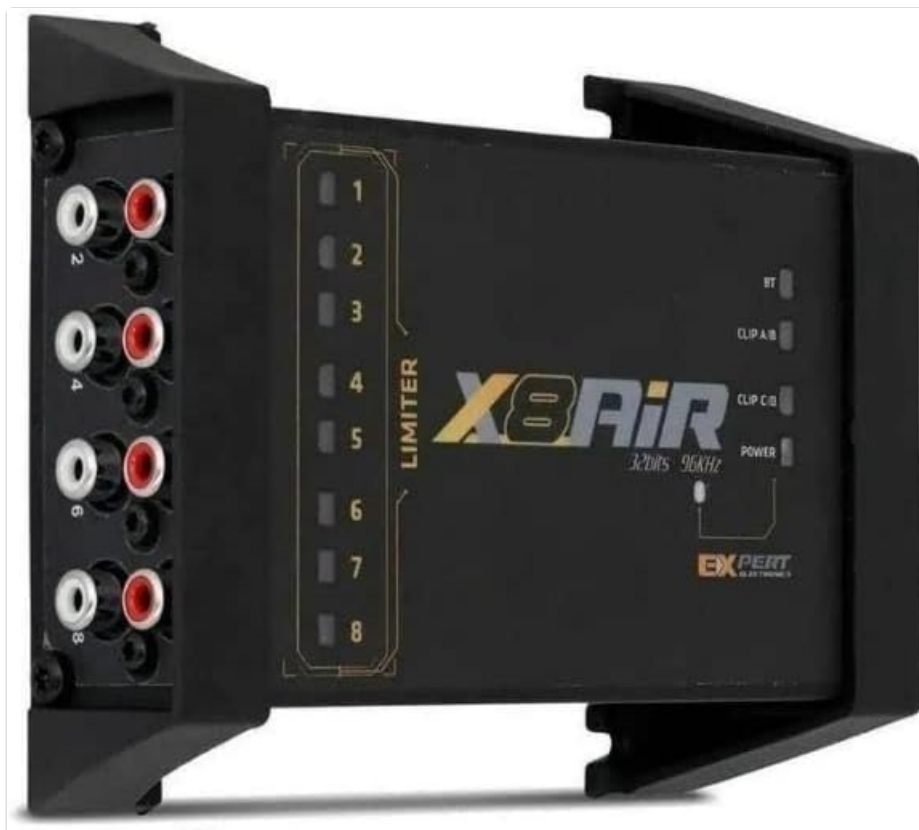
Figure 2: Side view of the EXPERT X8AIR DSP, illustrating the eight RCA output connections.
