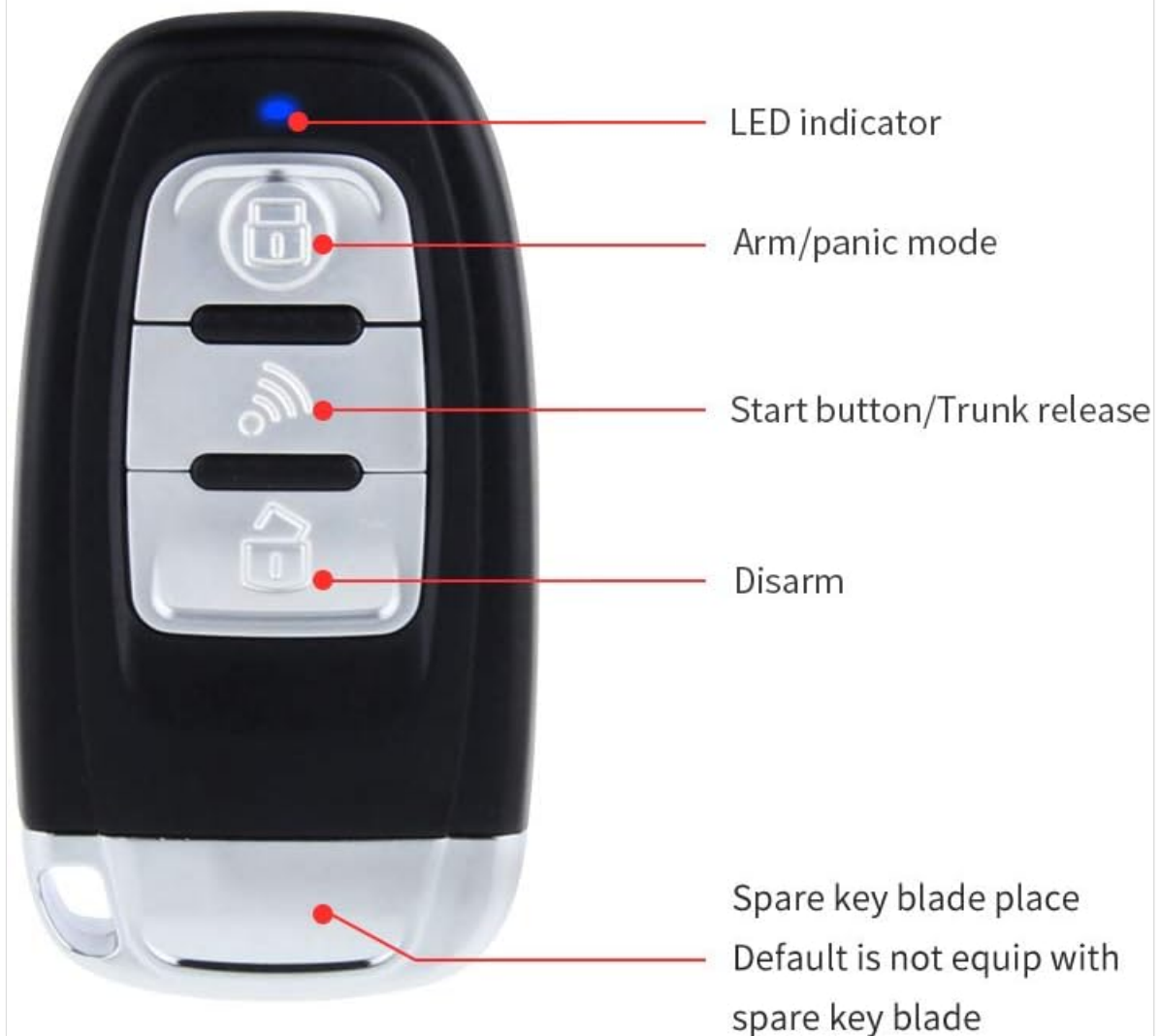
Figure 4.3: Diagram of the key fob buttons and their corresponding functions. The key fob features buttons for arm/panic, start/trunk release, and disarm, along with an LED indicator.
