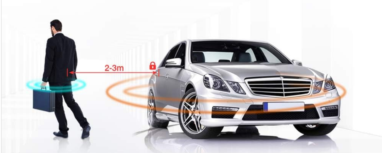
Figure 4.1: Illustration of the PKE automatic unlock function. The car unlocks when the key fob is within 1-2 meters.
