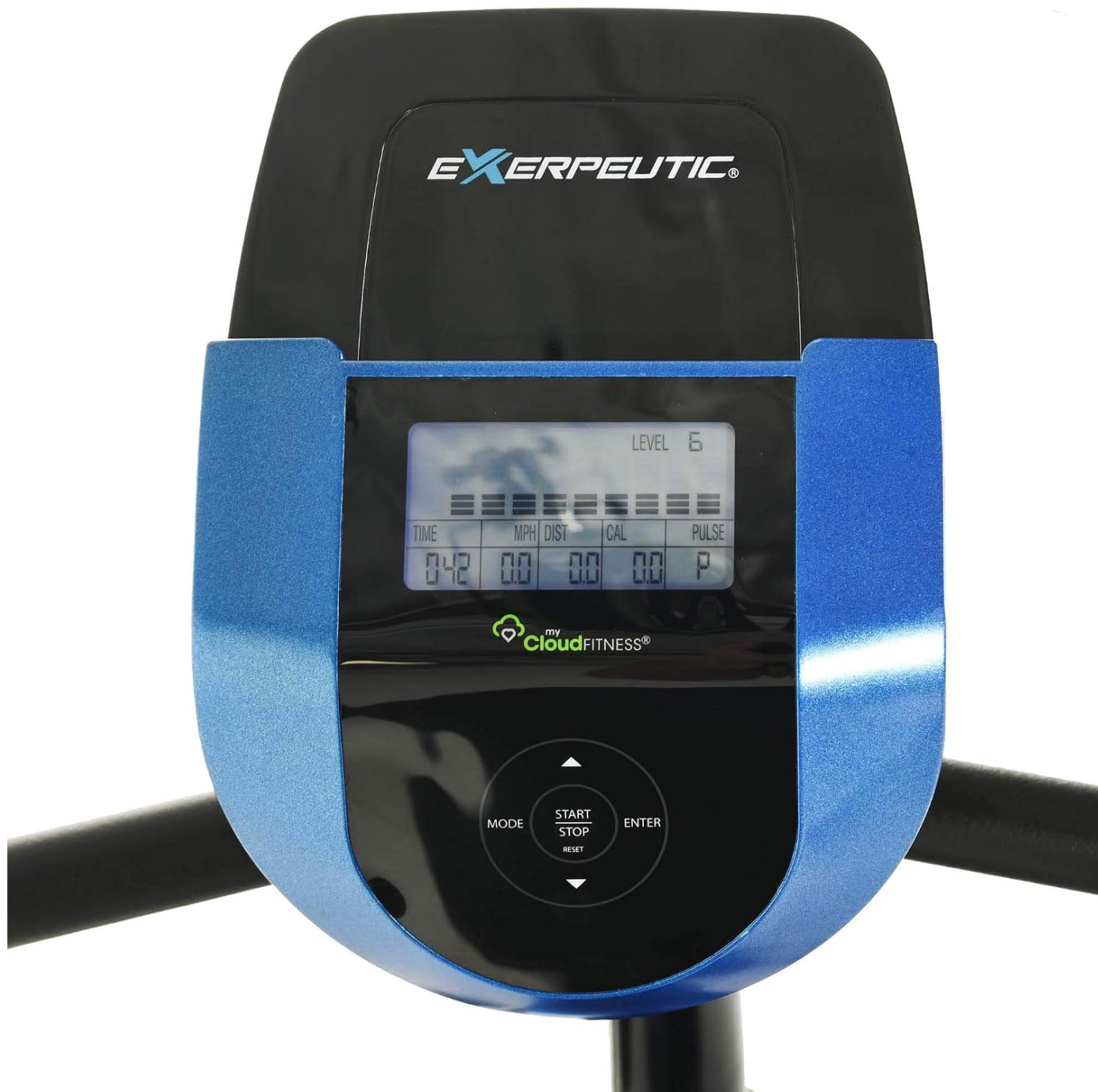
Figure 4.1: The console displays workout data such as Time, MPH/Distance, Calories, and Pulse. Buttons for MODE, START/STOP, and ENTER are located below the screen.
