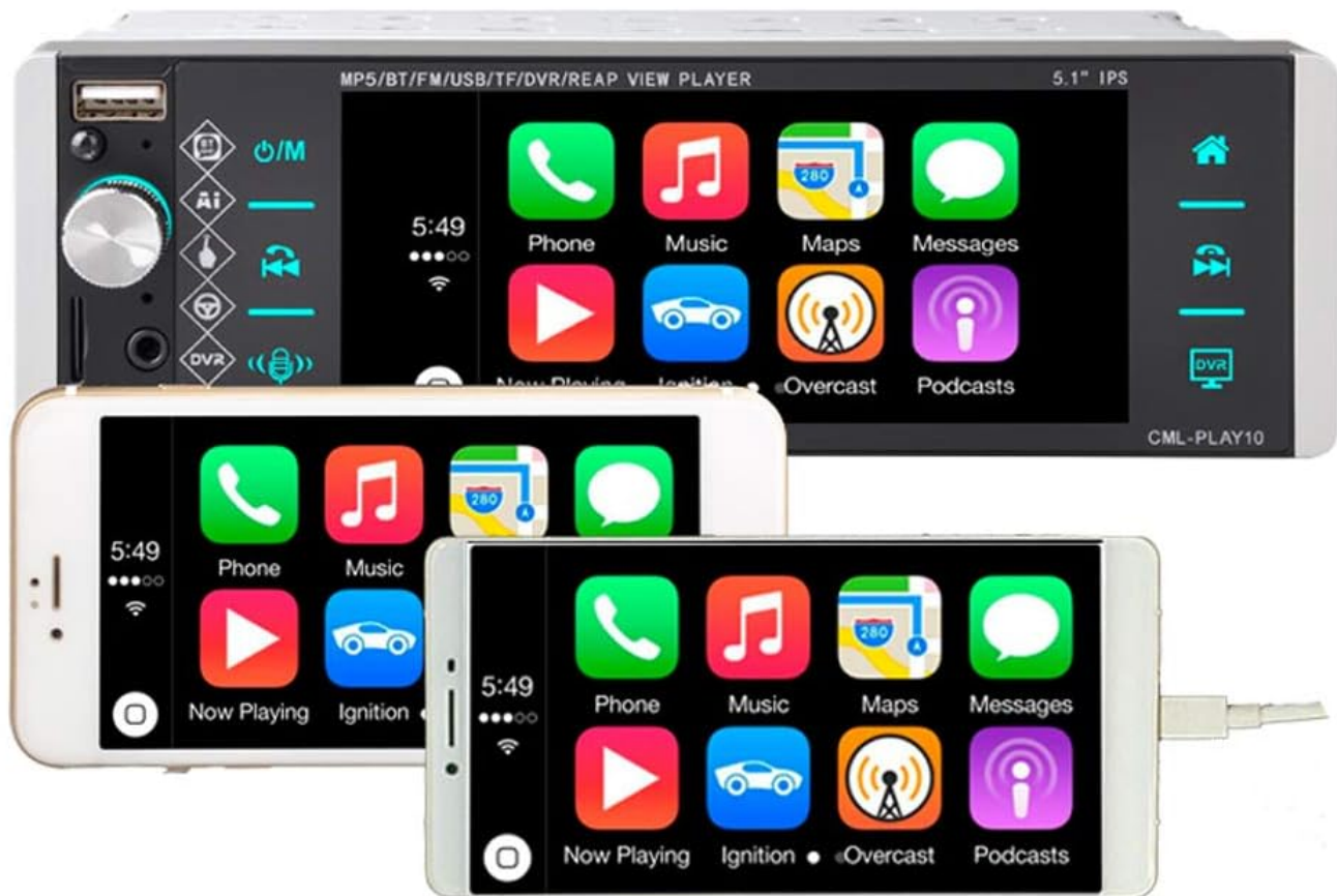
Image 6.5: The MirrorLink feature demonstrating two-way interconnection with both iOS and Android devices.
